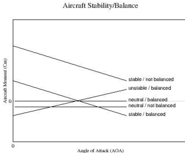
At this point it should be clear that there is no one term in the equations above, such as a lifting tail, that cause instability. It is the aerodynamic design, the combination of elements, that determine stability, and stability is only one aspect of a design.
